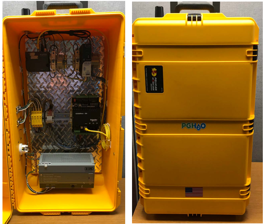
The portable SCADA sampling kit functions as a traveling laboratory for field testing and sampling.
