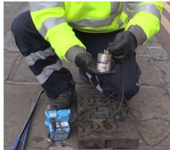
Consistent noise picked up by a logger helps to pinpoint the exact location of a leak.
