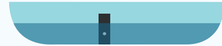
c) Following the event, the control orifice for a pond is partially opened to facilitate a slow draw down to maximize water quality benefits.
