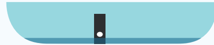
b) Prior to a storm event, the control orifice for a pond is opened to draw down the water level and increase storage capacity.
