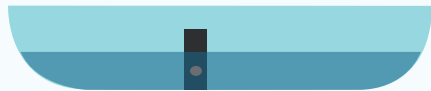
a) During dry weather, the control orifice for pond is closed to maximize water retention for recreation and habitat value.
